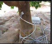
To determine the usefulness of innovative procedures for determining soil moisture temporal dynamics and soil-plant interactions using minimally invasive 3D micro-electrical and geophysical Electrical Resistivity Tomography (ERT.)
